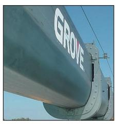
36 - 110 ft. (11 - 33.5 m) four section full power sequenced synchronized MEGAFORM™ boom designed for maximum vertical and lateral strength
