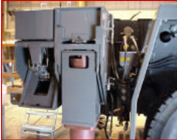
Rear outrigger box can be self-removed for roading
