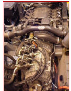
Chassis power is supplied by a 563 hp Mercedes diesel engine driving thru an Allison 7 speed automatic transmission
