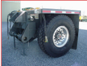
OPTIONAL 8 th axle pins on in place of rear box (shown with optional aluminum wheels)
