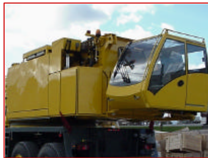
New Superstructure cab is located on right side for crane operation, and rotates to the rear for travel
