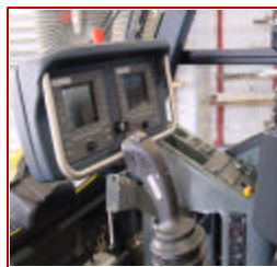
New Superstructure cab is located on right side for crane operation, and rotates to the rear for travel
