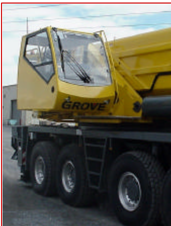
New Superstructure cab is located on right side for crane operation, and rotates to the rear for travel
