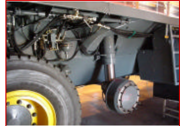
The exclusive Grove MEGATRAK independent suspension system allows all wheels to be on the ground at all times.
